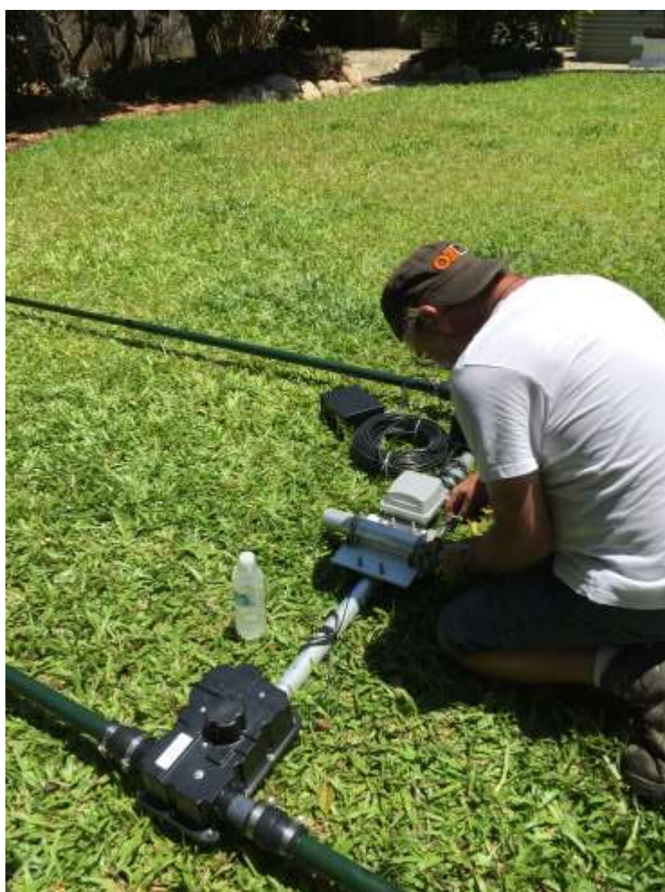
Figure 2. Helmut(VK4YKI) building an arm-strong rotator mechanism for turning the SteppIR 2el Yagi(s).
