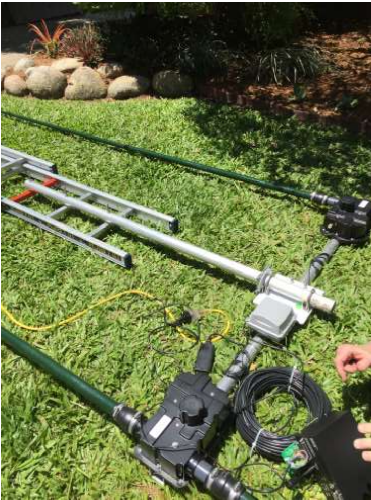
Figure 3. Testing the SteppIR 2el Yagi(s). Notice the 9m(29.5ft) ladder/Yagi interface mechanism.
